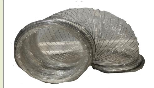
Flex Duct is a flexible ducting that is offered in clear (as seen in picture above) or silver. It can be used with negative air machines and other air movement applications. Comes in 25' sections which are 12" in diameter.
