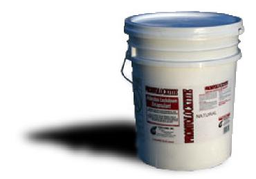
PRONTO LOCKTITE is an economical and efficient asbestos lockdown encapsulant. This is a ready to use product that is designed to lock down asbestos fibers in your work areas and help you pass even the most aggressive air tests. PRONTO LOCKTITE penetrates asbestos rapidly and completely. When it penetrates, it absorbs onto the individual fibers to lock them together, reducing the possibility of loose fibers from becoming airborne during the removal process.
